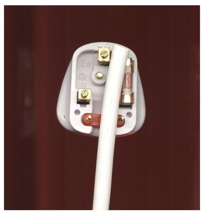
Hold the wire up to the plug, ensuring that the wire reaches the furthest terminal (the earth).
